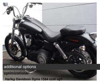
upchip Chiptuning 56kW/76HP » 66kW/90HP 123Nm » 140Nm
